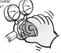
Operate the pressure adjusting screw to confirm the maximum service pressure can be obtained.
