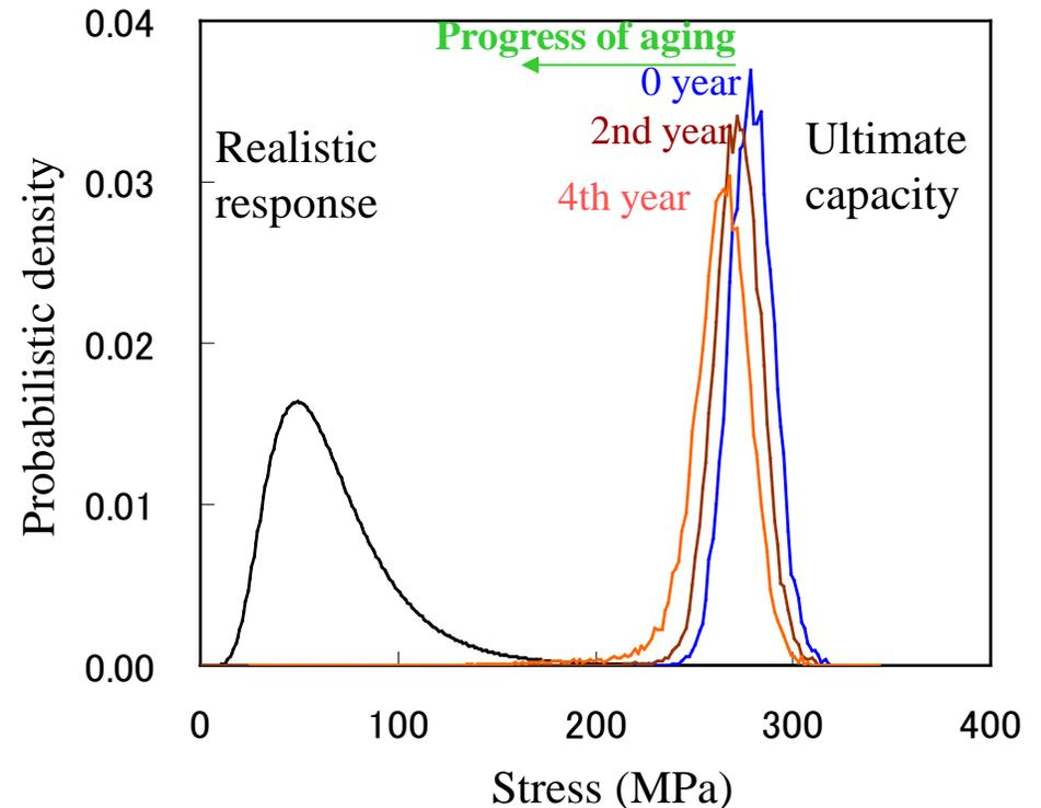
Failure probability considering seismic stress and probabilistic distribution of ultimate capacity
