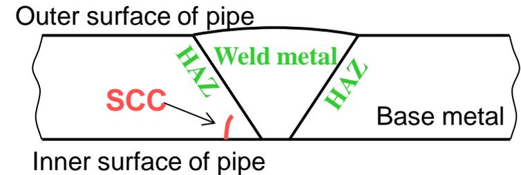
**SCC in a weld joint**
