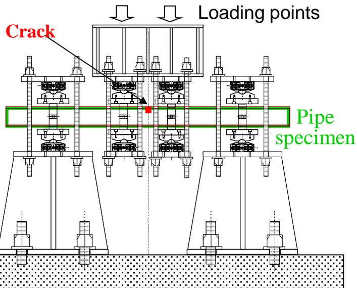
Experiment using seismic load and pipe specimen
