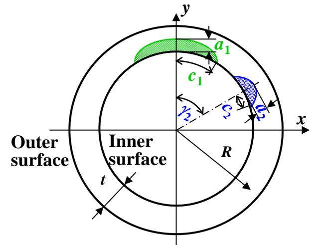
**Circumferential semi-elliptical surface cracks in weld joints**
