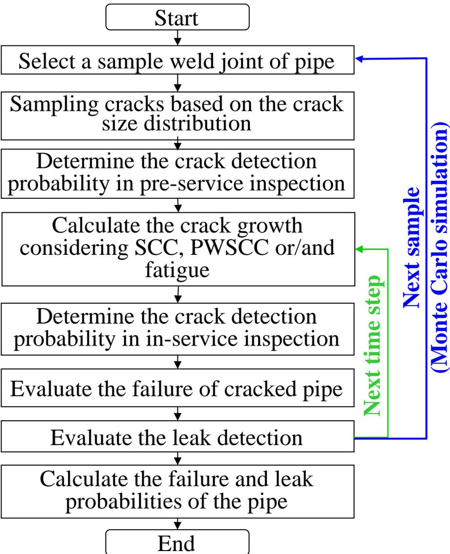
✓ In order to conduct seismic PRA or seismic safety evaluation for existing NPPs, a PFM analysis code for aged piping has been developed to evaluate failure probabilities and fragility curves of cracked pipes considering aging mechanisms and seismic loads.
