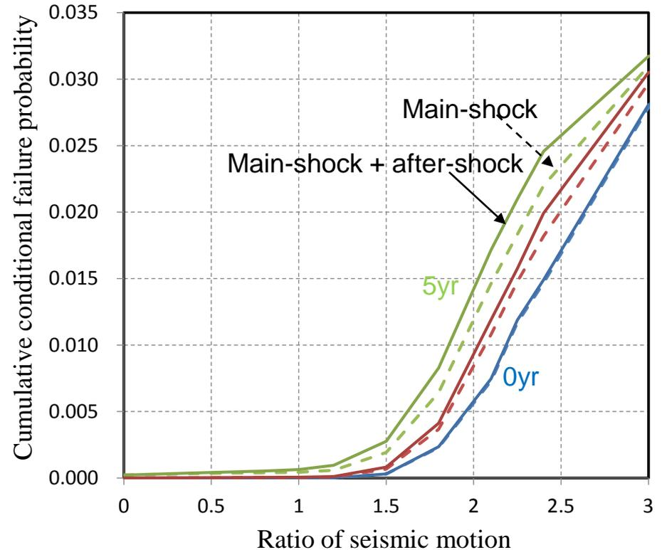
**Failure probability and seismic fragility curve with the effect of after-shock**
