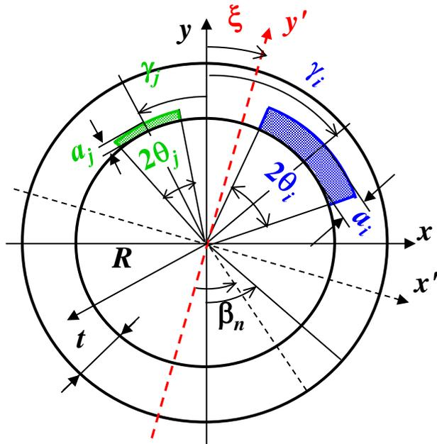
Pipe section with multiple cracks
