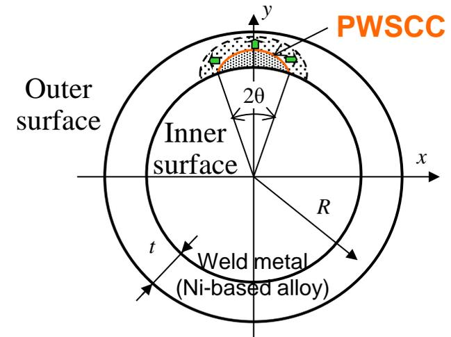
**Circumferential semi-elliptical surface cracks in weld joints**
