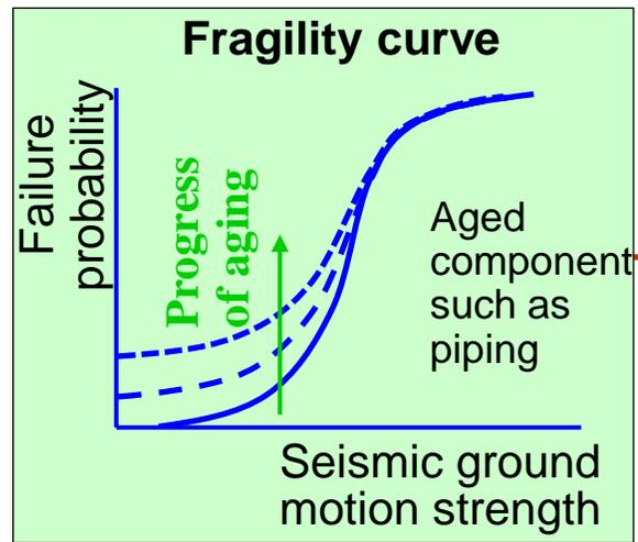
**Process of seismic PRA and failure probability considering age-related degradation**
