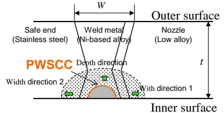
**Axial semi-elliptical surface cracks in weld joints**
