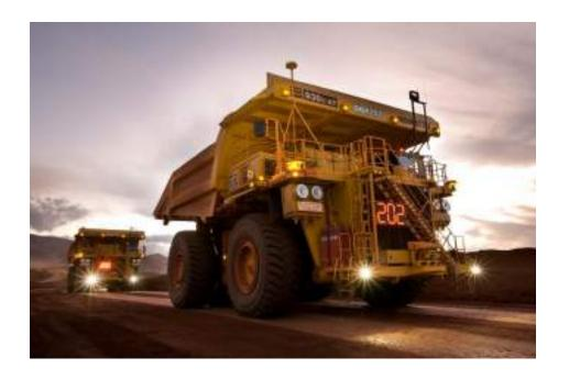
Earth moving machines are exposed to tough condition and less fuel consumption by reducing the weight by high tension steel is key issues
