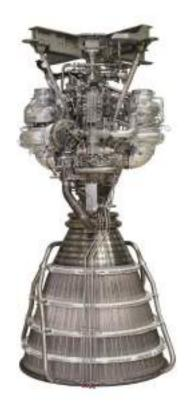
Engines for space vehicle are used under the severe condition from lowest to highest temperature because of the use of liquid oxygen and hydrogen as fuel
