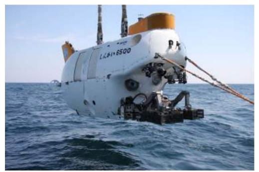
'Shinkai 6500' is the advanced submarine which could dive into the depth of 6500m
